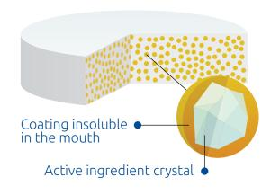
Active ingredient crystals are coated to obtain taste-masked particles with a diameter between 200 and 600 microns, ideal for suspensions, dispersible tablets, or chewable tablets. The coating is designed to be insoluble in the mouth but quickly soluble in the gastric environment, without interfering with bioavailability.
